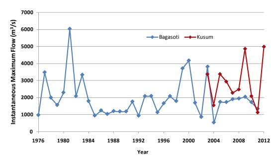
Figure 3. Instantaneous maximum discharge at Bagasoti and Kusum (Source: DHM)
